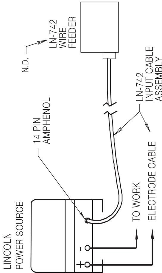
N.A. WELDING CABLE MUST BE SIZED FOR CURRENT AND DUTY CYCLE OF APPLICATION.
