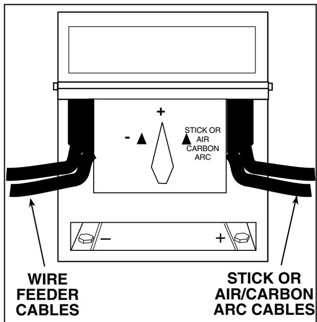
FIGURE C.1 - MULTI-PROCESS SWITCH
