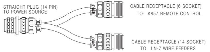
A “V” cable 12” (.30m) long to connect a K857 Remote Control (6 pin connector) with a wire-feeder (14-pin connector) and the machine (14-pin connector). If a remote control or amptrol is used alone the wire-feeder connection is then not used.
