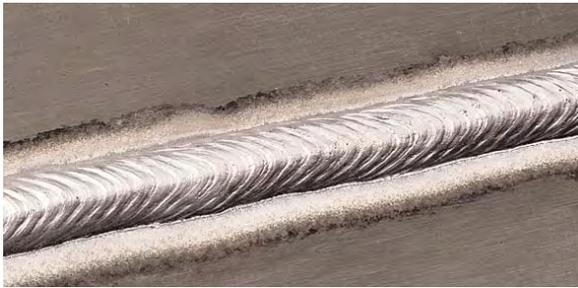
The pulsing frequency is adjustable. Changing the frequency modulation (or arc control) of the waveform changes the ripple spacing. Faster travel speeds may be achieved by using higher values of frequency modulation.
