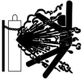
Gas under pressure is explosive. Always keep gas cylinders in an upright position and chained to the undercarriage or a stationary support. See American National Standard Z-49.1, "Safety In Welding And Cutting", published by the American Welding Society.
