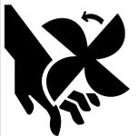
1.d. Keep all equipment safety guards, covers and devices in position and in good repair. Keep hands, hair, clothing and tools away from V-belts, gears, fans and all other moving parts when starting, operating or repairing equipment.
